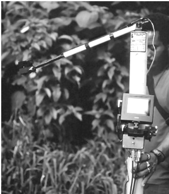
Fig. 1. Telescoping, intra-cavity video probe.
